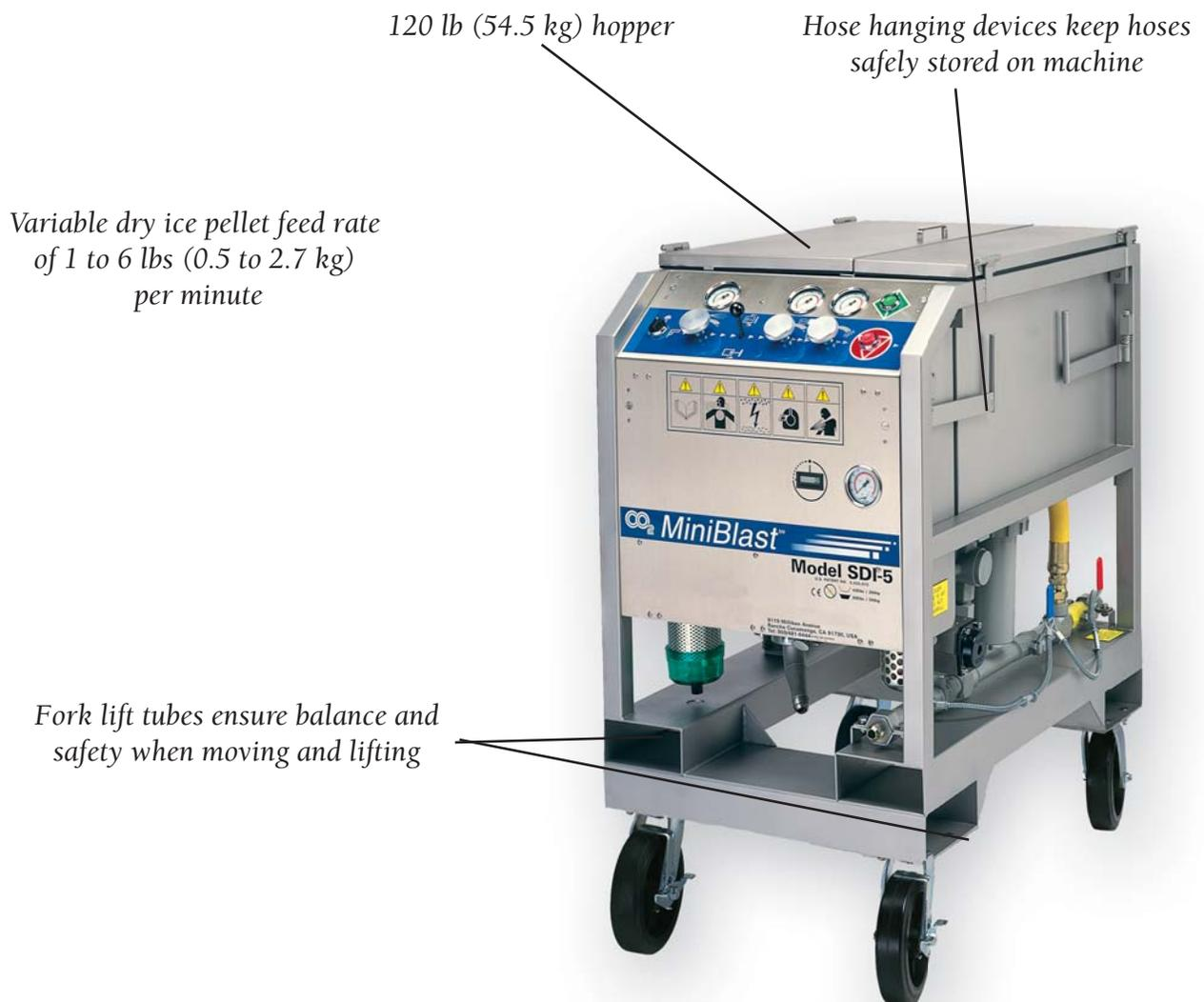
The dry ice blasting system includes one length of dry ice blast applicator and hose assembly, one length of air hose, customer-specified nozzle (with appropriate handle if applicable) and stinger.
